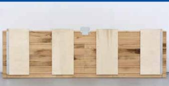
Underneath each floor panel is fitted four sheets of birch plywood, 12 mm thick. These give the panels a great deal of strength and durability. The panels are reinforced in each end with aluminum profiles.
